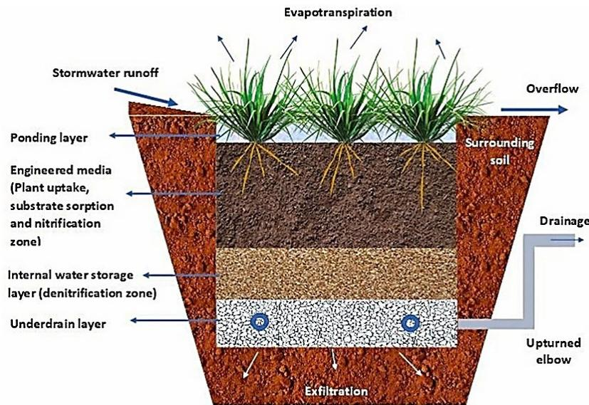
**Figure 41.** From “Bioretention systems for stormwater management: Recent advances and future prospects” by Vijayaraghavan *et al.*, 2021, Journal of Environmental Management, 292, p. 2. Schematic representation of a bioretention container. These systems are useful in urban areas with limited space and have multiple layers of soil media.
