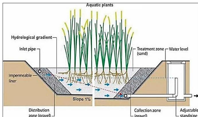
**Figure 44.** From “Constructed wetlands for wastewater treatment in cold climate — A review” by Wang *et al.* 2017, *Journal of Environmental Sciences*, 57, 293-311. Schematic representation of treatment wetlands. These are passive systems that help remove pollutants while providing habitat to wildlife and aesthetic value to the landscape.
