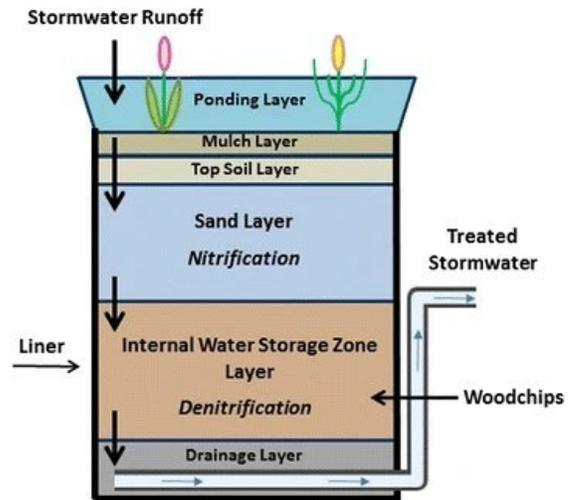
**Figure 45.** From “Application of denitrifying wood chip bioreactors for management of residential non-point sources of nitrogen” by López-Ponnada *et al.*, 2017. *Journal of Biological Engineering*. 11(1), 1-14. Schematic representation of a woodchip bioreactor. This system provides the proper environment to promote the denitrification of wastewater.
