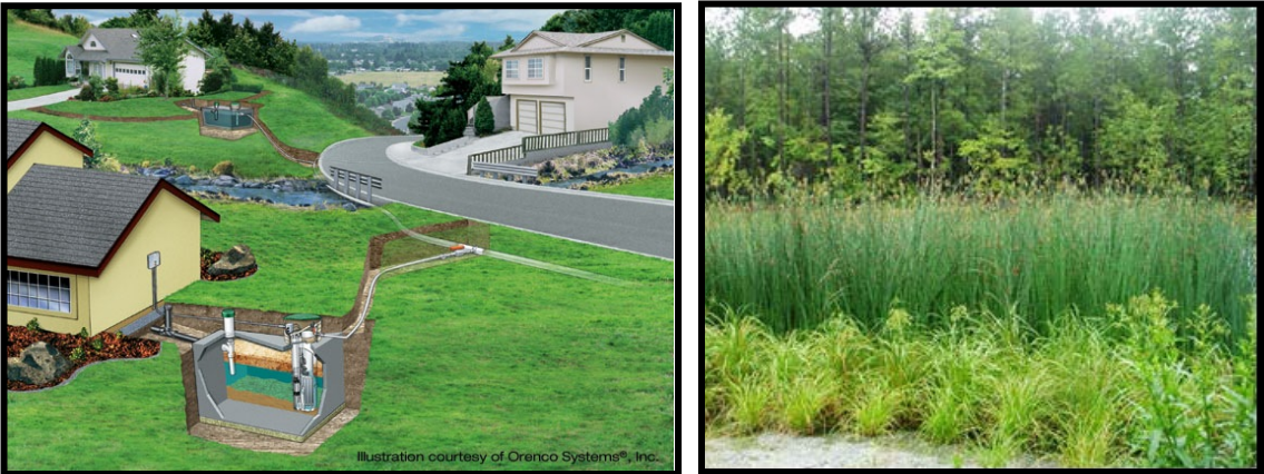
Figure 19. Pump and treat system effluent is pumped from homes to a constructed wetland or landscaped area
